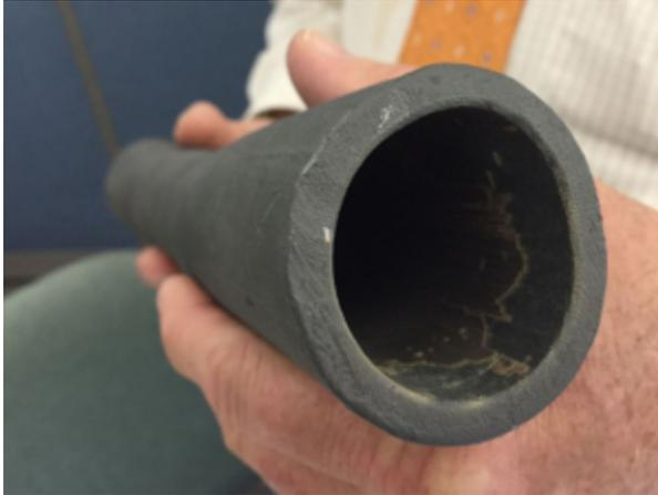
Be sure to scratch test your pipes in multiple areas. It is not uncommon to have more than one type of piping on your water line.
